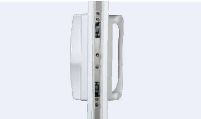
TWIN-POINT LOCK Standard on all doors. This heavy-duty latch system locks at two points on the door frame and includes an anti-slam mechanism for added safety.
